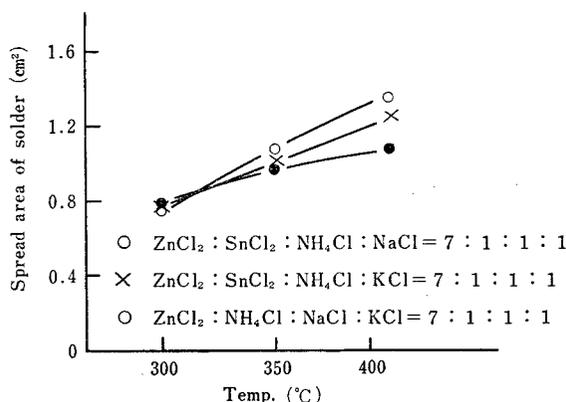
Fig. 5. Spread area of Sn-Pb eutectic solder with various quarternary system fluxes on SUS27.
