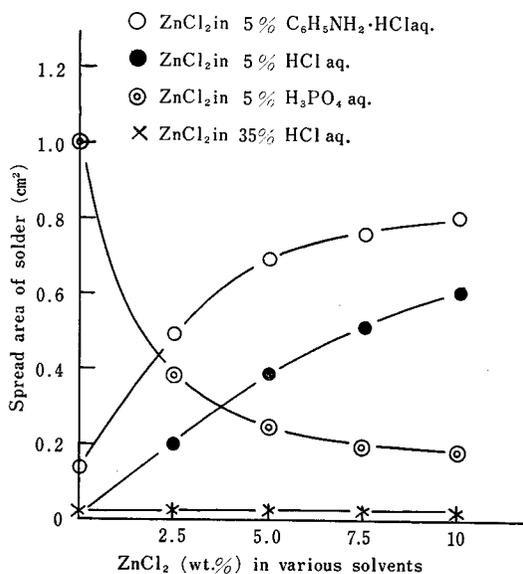
Fig. 10. Effect of  $\text{ZnCl}_2$  content in various solvents on spreadarea of Sn-Pb eutectic solder at  $300^\circ\text{C}$ .
