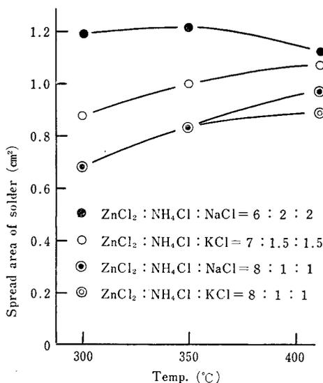
Fig. 4. Spread area of Sn-Pb eutectic solder with ternary system flux which don't contain  $SnCl_2$  on SUS27 plate.
