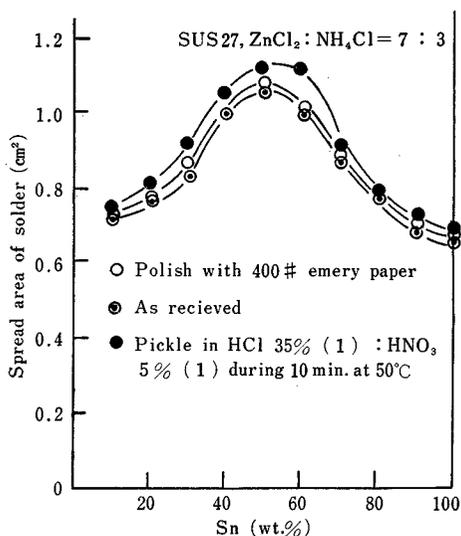
Fig. 11. Effect of surface conditions on the spread area of Sn-Pb solders at 300°C.
