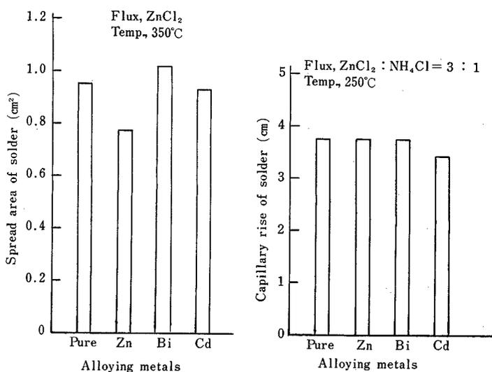
Fig. 12. Relation between the spread area or capillary rise and 2 wt. % other alloying metals added to Sn-Pb eutectic solder.
