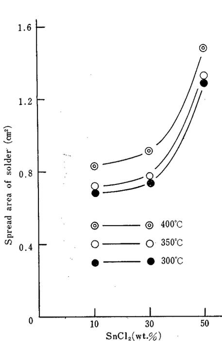
Fig. 2. Spread area of Sn-Pb eutectic solder on SPC1 plate with  $ZnCl_2$ - $SnCl_2$  binary fluxes.
