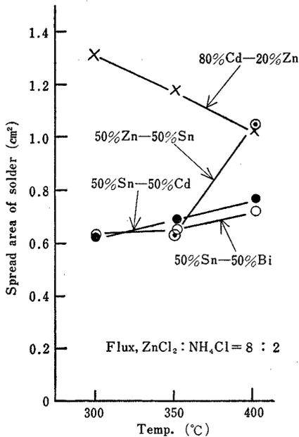
Fig. 8. Spread area of various binary system solders on SUS27 plate.
