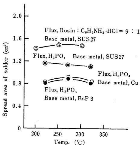
Fig. 7. Spread area of Sn-Pb eutectic solder on various base metals.
