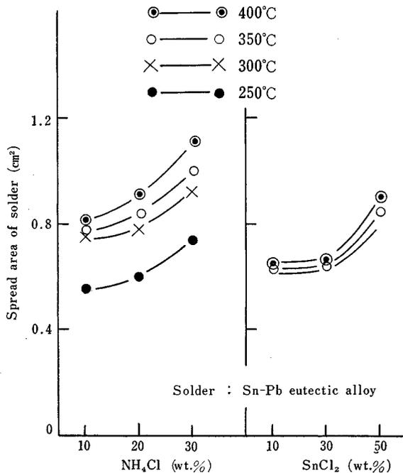
Fig. 1. Spread area of Sn-Pb eutectic solder with  $ZnCl_2-NH_4Cl$  and  $ZnCl_2-SnCl_2$  binary fluxes on SUS 27 plate.
