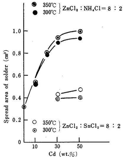
Fig. 9. Spread area of Pb-Cd solders on SUS27 plate.
