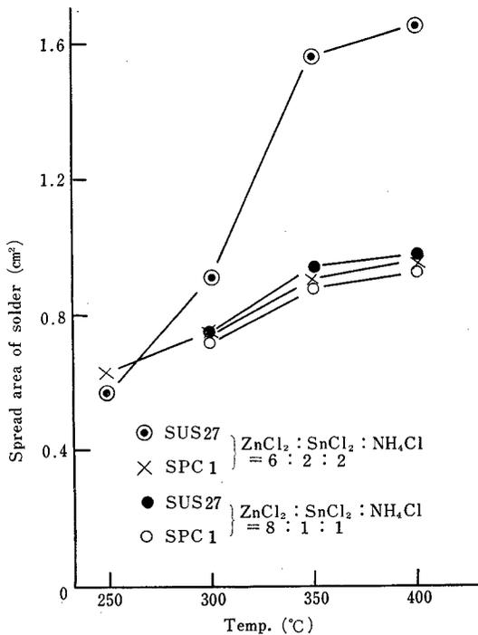
Fig. 3. Spread area of Sn-Pb eutectic solder with  $ZnCl_2$ - $SnCl_2$ - $NH_4Cl$  ternary fluxes on SUS 27 and SPC1 plates.
