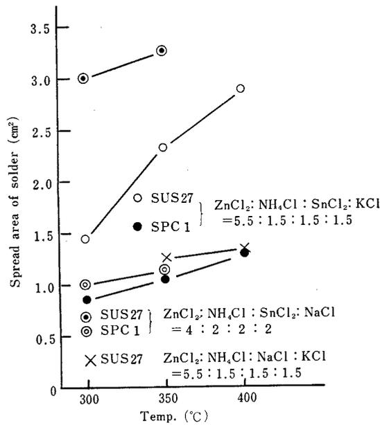
Fig. 6. Spread area of Sn-Pb eutectic solder with quaternary fluxes on SUS27 and SPC1 plates.
