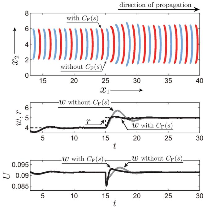
FIG. 8. Control performances of the PI control system without the feed-forward compensator  $C_F(s)$  as shown in Fig. 1 and with the feed-forward compensator as shown in Fig. 7.
