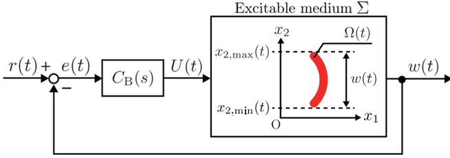
FIG. 1. Feedback system with PI control [23].
