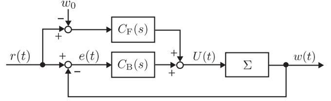
FIG. 7. Control system with feed-forward compensation.
