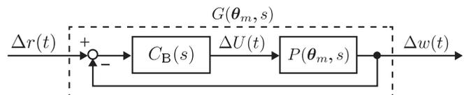
FIG. 3. Block diagram of a linear system around the steady state of the PI control system.
